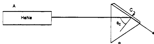
Figure 3. Apparatus used for refractive index measurements. 36 HeNe laser (A) illuminates polymer film (C)-prism (B) interface. Rotation of prism until total internal reflection occurred allowed calculation of critical angle \theta_c .
